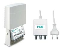
3-input (III+DAB, UHF, UHF) pole mount amplifier with 28dB gain and output level up to 116dBµV in UHF band, separate VHF/UHF amplifications, independent gain adjustments (0-15dB) for each input and low noise figure. 2 outputs and builtin 5G and 4G LTE 694MHz filter. Power supply included in the package.
